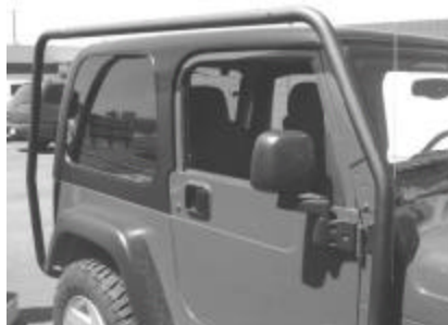
Figure 6 – Uprights installed, DO NOT TIGHTEN.
