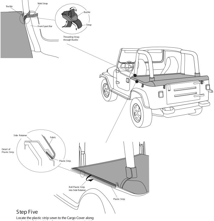
each side of the vehicle. Start at one end on each side and roll the plastic strip into the Side Retainers.
