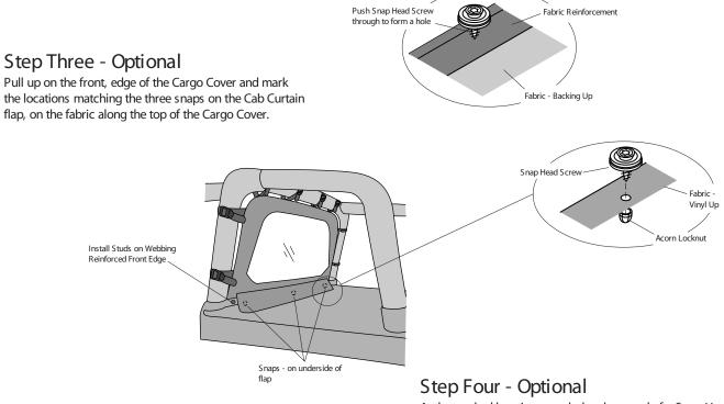
At the marked locations, push the sharp end of a Snap Head Screw through the Cargo Cover from the vinyl side so that the snap is on top of the vinyl. Thread an Acorn Locknut over the pointed end of the Snap Head Screw. Snap the Cargo Cover and the Cab Curtain together with the three snaps.
