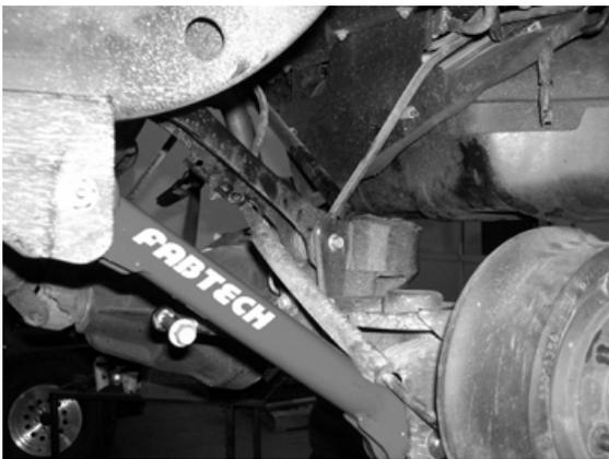
33. If installing Fabtech's optional upper link kit, install rear upper at this time. See instructions included in Fabtech's upper link arm kit.
