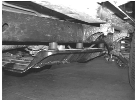
23. Reinstall the front driveline, using factory hardware.
