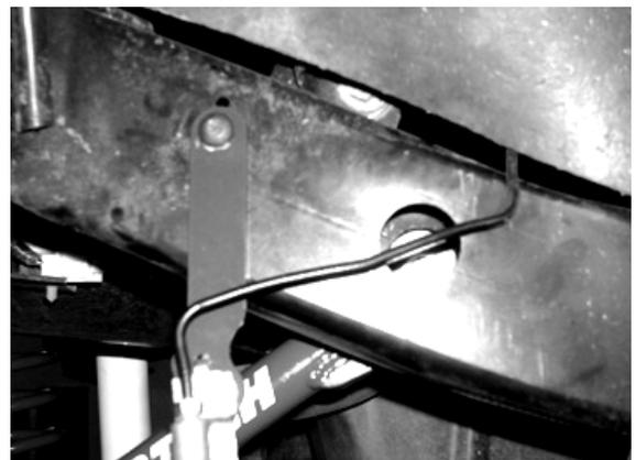
12. Locate the new Fabtech bump stop FT50027. Install into factory pocket by pushing bump stop in until fully seated. SEE PHOTO BELOW.
