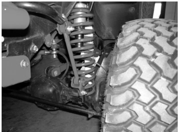
43. Using a grease gun, grease all grease fittings in the new Fabtech Link Arms.
