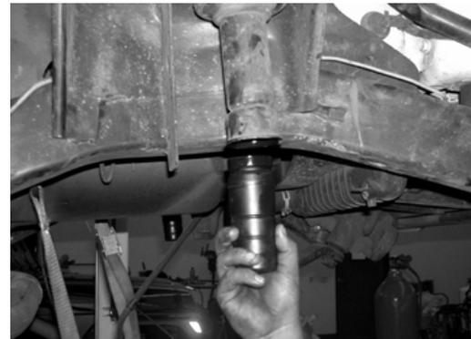
20. Locate the new Fabtech lower Aluminum bump stop FT50052. Using a drill, drill a 5/16" hole through the center of the lower coil spring mount. Using the supplied 5/16" x
