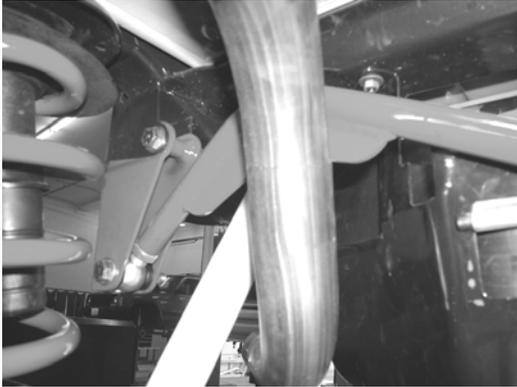
62. Working for the driver side of the truck, locate the three outer tabs on the Fabtech Subframe. With a sanding wheel, clear the power coat from the tabs and paint from the frame. Using a Mig Welder, weld the tabs to the frame. Once the weld has cooled spray paint all raw metal areas of the frame to prevent rust. Repeat on the passenger side of the truck. SEE PHOTO BELOW.
