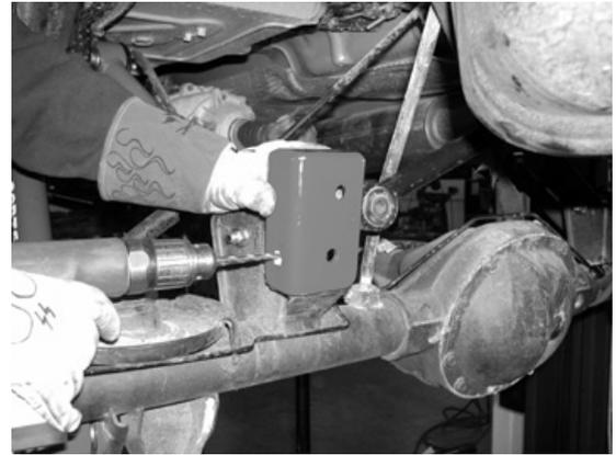
59. Locate the Fabtech upper frame Trac bar bracket FT50054. Using the supplied 1/2" x 1 1/4" bolt, and washer and 1/2" x 3 1/2" bolt, nut, and washer attach the bracket to the frame. Torque both bolts to 75 ft. lbs. SEE PHOTO BELOW.
