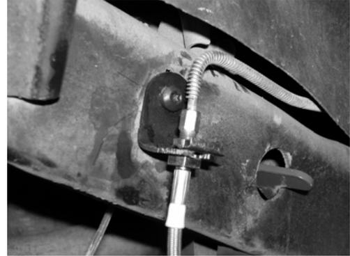
18. Locate the supplied brake line retaining spring and Adel clamp. Using a drill, drill a guide hole directly below the brake line bracket on the frame. Attach the spring to the frame using the supplied 5/16" self tapping screw. Attach the other end on the spring to the brake line using the supplied Adel clamp and 1/4" bolt, nut, and washer. SEE PHOTO BELOW.
