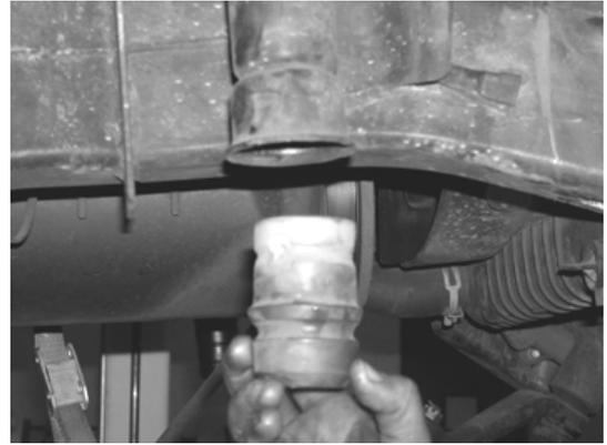
44. Working from the driver side of the truck, remove and discard the lower link arm. Discard the factory hardware. SEE PHOTO BELOW.
