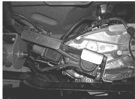
29. Locate the factory pitman arm, disconnect the inner tie rod end from the pitman arm, remove the pitman arm with a pitman arm puller and discard. Locate the new Fabtech drop pitman arm FT50015 and install onto the steering box using the factory nut and washer. Torque nut to 185 ft lbs. Reconnect the inner tie rod end using factory hardware. Torque to 45 ft lbs.
