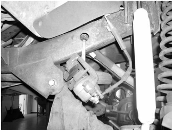
5. Remove the front shocks and discard. Save the factory lower shock hardware, discard the upper hardware.
