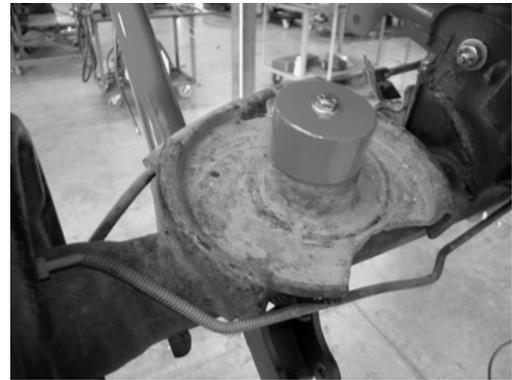
51. Locate the previously remove brake line and e-brake cable from the upper link arm. Reattach to the Fabtech link arms using factory hardware on the passenger side and the supplied 5/16" bolt, nut, and washer on the driver side. SEE PHOTO BELOW.
