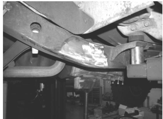
46. Locate the shock mount on the axle. Using a die grinder with a cut off wheel cut shock mount completely from the
