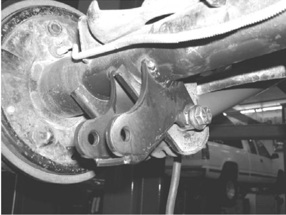
47. Locate the factory upper link arm, remove and discard link arm and save hardware.
