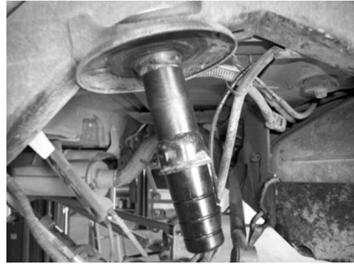
50. Locate the new lower bump stop FT50052. Using a drill, drill a 5/16" hole through the center of the lower coil spring mount. Using the supplied 5/16" x 2" bolt, nut, and washer attach to the lower coil mount. SEE PHOTO BELOW.
