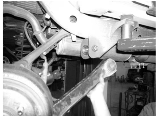
45. Locate the factory lower link arm frame pocket, using a die grinder with a cutoff wheel cut the link arm pocket from the frame. Clear bracket completely from the frame. SEE PHOTO BELOW.
