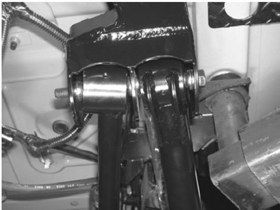
49. Locate the upper bump stop cup, remove and discard bolt. Locate the bump stop drop spacer FT50062 using the supplied 10mm-1.5mm x 105mm bolt and washer install the spacer between the bump stop cup and upper coil seat.
