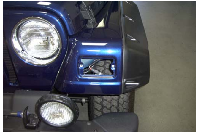
Photo #1 – Front Marker Light Cover Removed
