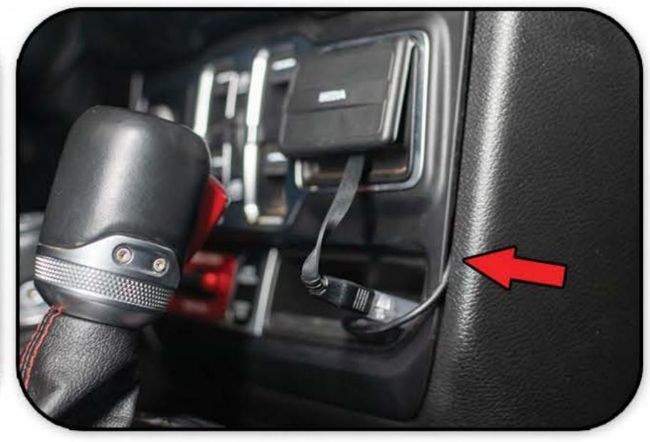
REPLACE THE SCREEN TRIM AND THE CLIMATE CONTROL MODULE. THE USB CABLE WILL PASS FROM BEIND THE PANEL.
