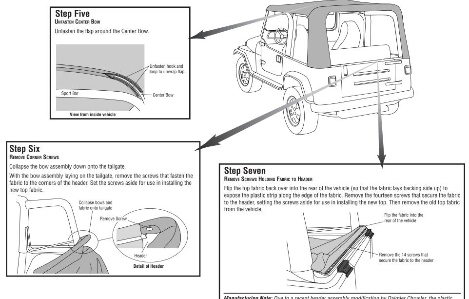
**Manufacturing Note:** Due to a recent header assembly modification by Daimler Chrysler, the plastic strip on the windshield header may have 8 screw locations instead of 14. Both attachment numbers of screws will securely fasten the header and perform as the original design was intended.
