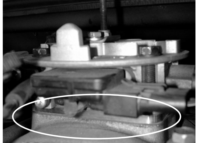
b) Install throttle body spacer and gaskets under throttle body. Tighten throttle body bolts to 9 ft-lbs.
