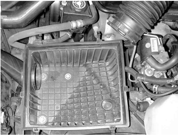
e) Remove the air cleaner cover and air filter.
