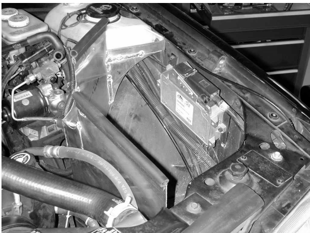
f) Place heat shield in bay as shown.
