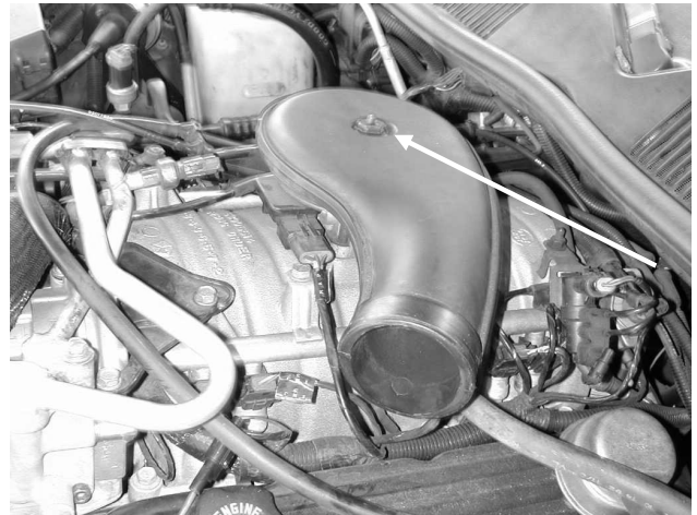
l) Remove plastic nut, and remove plastic housing.
