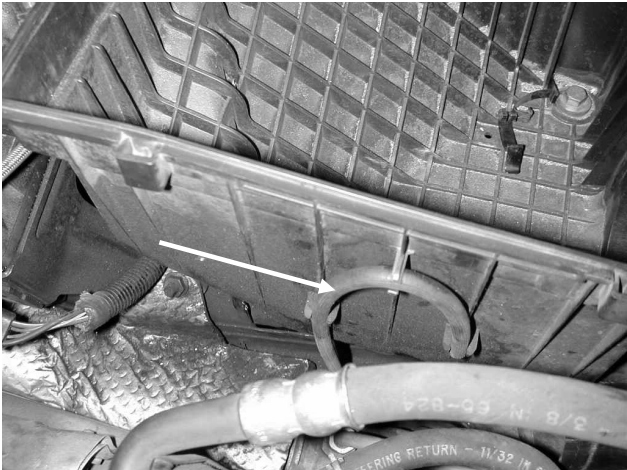
g) Unclip small breather hose from the side of the lower air box and then remove lower air box.
