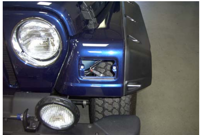
Photo #1 – Front Marker Light Cover Removed
