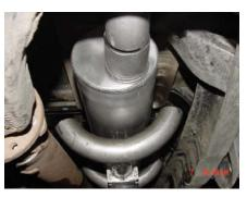
INSTALL MUFFLER #B ONTO HEADPIPE 1-1/2" TO 2" WITH THE INLET FACING THE MOTOR. ROTATE MUFFLER UNTIL THE OUTLET IS AT THE 6 O'CLOCK POSITION. THE INLET OF THE MUFFLER IS LOOKING INTO THE LOUVERS.
