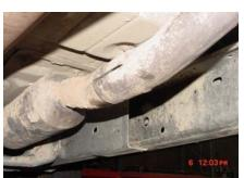
TO REMOVE STOCK EXHAUST UNBOLT THE CLAMP LOCATED JUST BEHIND THE CONVERTER. YOU MAY NEED TO HEAT IT UP FOR EASIER REMOVAL. CUT STOCK TAILPIPE OFF BEHIND THE MUFFLER & REMOVE. LEAVE ALL RUBBER GROMMETS ON THE HANGER. USE WD-40 TO AID IN THE REMOVAL OF EXHAUST AND
