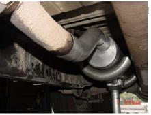
INSTALL HEADPIPE #A ONTO STOCK PIPE 1-1/2" TO 2". USE CLAMP #H TO SECURE THEM TOGETHER. DO NOT TIGHTEN. OUTLET OF PIPE SHOULD BE AT THE 12 O'CLOCK POSITION.
