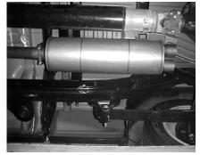
2. INSTALL HEADPIPE # A AND SECURE IT WITH CLAMP # G. NEXT **INSTALL MUFFLER # B WITH THE** INLET TOWARDS THE MOTOR. INLET HAS LOUVERS INSIDE FACING TOWARDS THE MOTOR. USE A JACK STAND TO SUPPORT THE MUFFLER. USE CLAMP # G TO SECURE MUFFLER TO THE STOCK PIPE, DO NOT TIGHTEN, INSTALL BAND CLAMP # J INTO RUBBER GROMMET AND INSERT WELDED HANGER. ATTACH WITH BOLT KIT # K. INSTALL # H HANGER TO THE PASSENGER SIDE MUFFLER OUTLET WITH VERTICAL BAR OF THE HANGER TOWARDS PASSENGER SIDE.
