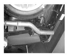
3.INSTALL PASSENGER SIDE OVERAXLE PIPE #C INTO MUFFLER AT LEAST 1 ½" NO MORE THAN 2". ATTACH WITH HANGER # H AND CLAMP # G.
