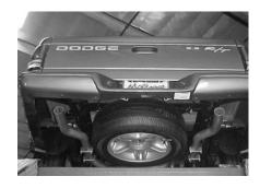
5. INSTALL EXIT PIPE # F TO OVERAXLE PIPES USE CLAMP # G TO SECURE THEM. DO NOT TIGHTEN. ADJUST PIPE TO THE RIGHT ANGLE AND CUT TO LENGTH. IF YOUR VEHICLE HAS A SWAY BAR YOU MAY HAVE TO TRIM THE FACTORY BOLT ON PASSENGER SIDE INSTALL CLAMP # G TO HANGER # I ON BOTH SIDES TO HOLD UP YOUR TAILPIPES.
