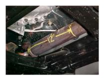
**TO REMOVE STOCK** EXHAUST MEASURE 12" FROM YOUR CATALATIC CONVERTER BACK **TOWARDS THE REAR** AND CUT HERE. NOW CUT OFF YOUR STOCK TAILPIPE JUST BEHIND THE MUFFLER AND REMOVE.LEAVE ALL RUBBER GROMMETS ON THE HANGER. USE WD-40 TO AID IN **REMOVAL OF** EXHAUST AND HANGERS.
