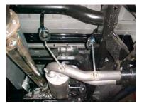
**INSTALL MUFFLER** ASSEMBLY #A ONTO STOCK PIPE 1-1/2" TO 2". SLIDE WELDED HANGERS INTO RUBBER **GROMMETS YOU** MAY NEED TO ADJUST WELDED HANGERS TO FIT INTO YOUR GROMMETS. USE A JACKSTAND TO SUPPORT YOUR MUFFLER. USE CLAMP #B TO SECURE IT TO YOUR HEADPIPE. DO NOT
