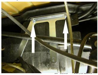
**Step 5:** On each side insert one of the 7/16-14 hex head bolts with a flat washer into the chassis through the larger of the holes shown below. Then position it with the threads facing downward through the smaller hole. If your TJ doesn't have these smaller holes from the factory, they will have to be drilled. Go to the next step.
