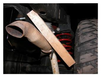
**Step 9:** You may find that you need additional exhaust system clearance as shown in the photo below left. Simply bend the exhaust hanger bracket shown below right to gain this clearance. You can also remove the threads that are protruding past the nut with a hacksaw.
