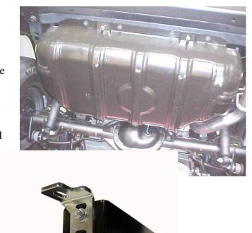
**Step 2:** Loosely attach both rear mounting brackets to the skid plate using the 5/16-18x1.0" carriage bolts, 5/16-18 nuts, and washers provided. The bolts should be installed from the inside of the skid plate. The longer bracket is installed on the passenger side of the vehicle to reach over the exhaust pipe.
