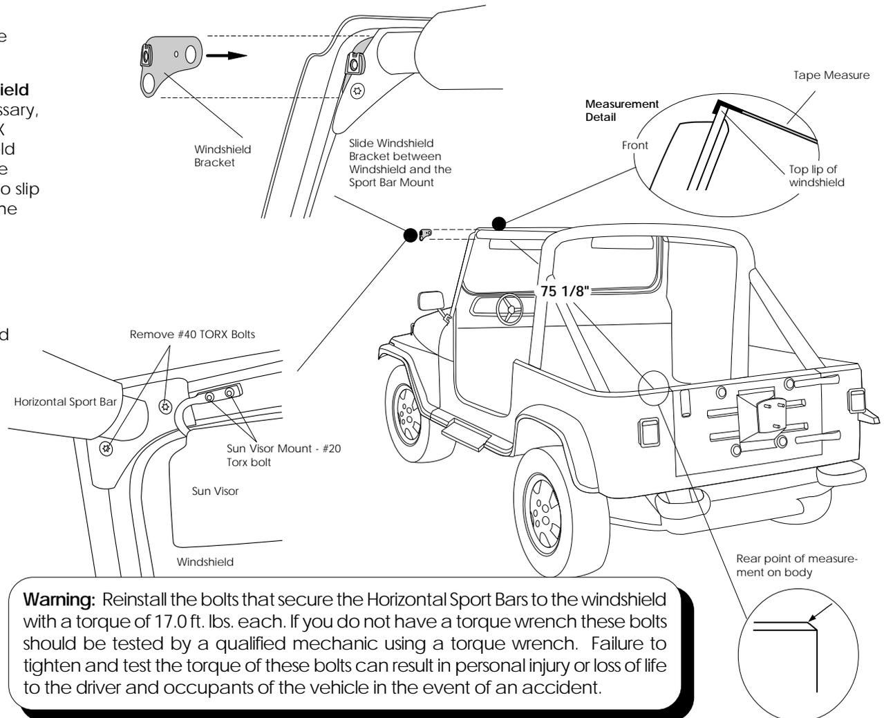
**Warning:** Reinstall the bolts that secure the Horizontal Sport Bars to the windshield with a torque of 17.0 ft. lbs. each. If you do not have a torque wrench these bolts should be tested by a qualified mechanic using a torque wrench. Failure to tighten and test the torque of these bolts can result in personal injury or loss of life to the driver and occupants of the vehicle in the event of an accident.
