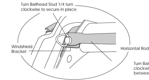
Turn Bailhead Stud 1/4 turn clockwise so pin catches between prongs on bracket
