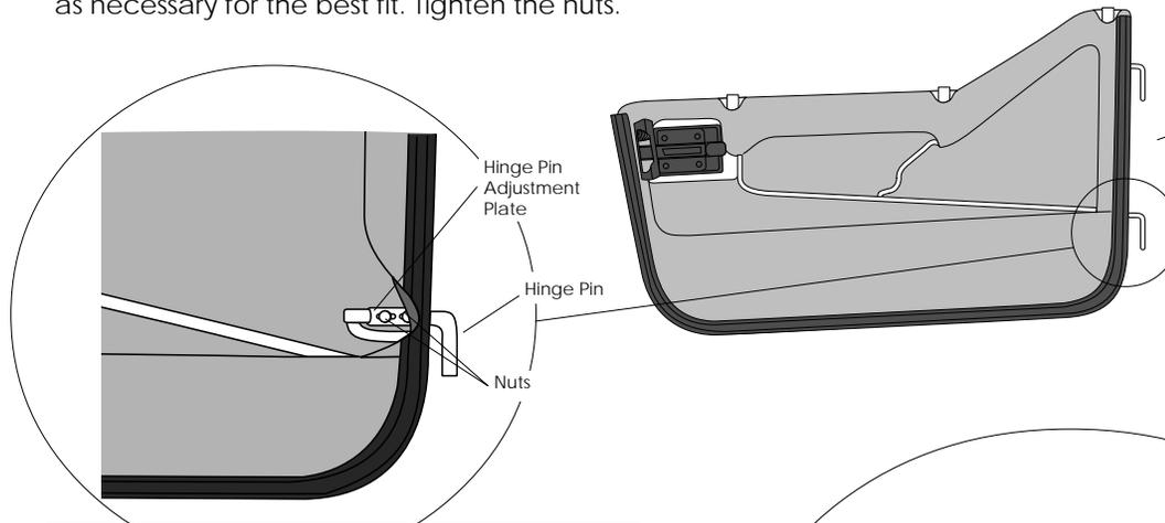
**Note:** If the lower door pivot does not provide enough adjustability for correct latch adjustment (the door does not latch properly), follow the instructions in the enclosed spacer kit.
