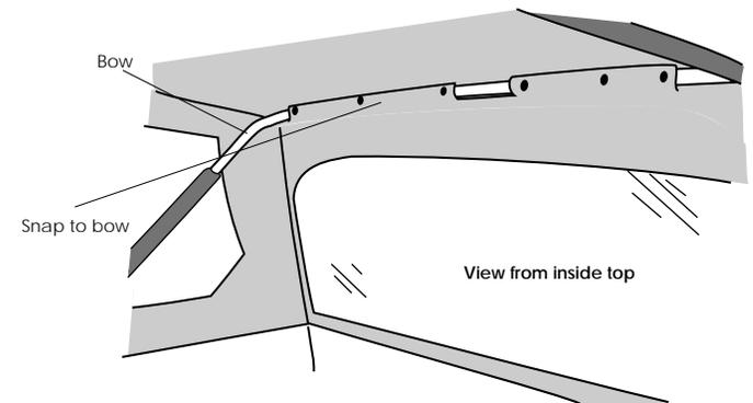
**Note:** If the snaps don't appear to line up, push the rear bow forward to relieve the pressure on the bow. This will allow the snaps to line up more easily.
