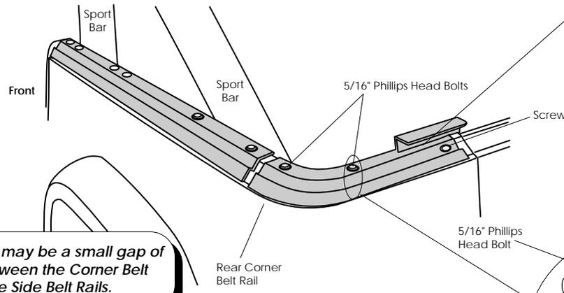
**Note:** There may be a small gap of +/- 1/4" between the Corner Belt Rails and the Side Belt Rails.
