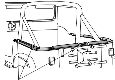
Leave packing tape on Bow Assemblies until front holes of Bow Mounts are secure
