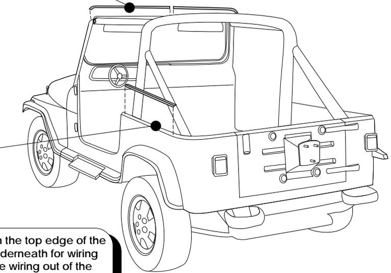
**Caution: When drilling in the top edge of the vehicle body, check underneath for wiring for the rear lights. Pull the wiring out of the way before drilling.**
