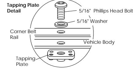
**Caution:** When drilling in the top edge of the vehicle body, check underneath for wiring for the rear lights. Pull the wiring out of the way before drilling.
