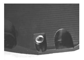
When draining oil, use bottom drain plug. If you remove the cover you have to readjust the shifter.
