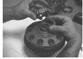
Install your bearings and shims in accordance with your MSM. Note: installation kit not included – bearings, shims, etc.
