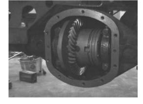
Check your pattern in accordance with your MSM. Note: gear set up should be done by a certified mechanic
