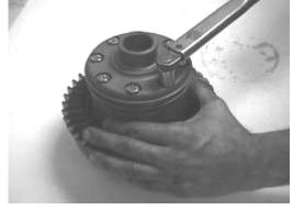
Torque  $\frac{1}{4}$  bolts to 12 FT LBS. Note: when tightening, tighten the bolts in the following pattern: 1-5-7-3-8-4-6-2
