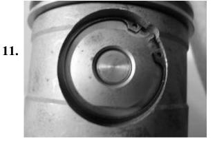
Install the snap ring into the groove. Make sure snap ring is fully seated into groove.
