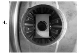
Rotate the carrier with opened end facing out so that you can install the c-clips.
