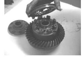
Install locking ring gear with gears facing engagement with locking side gear
