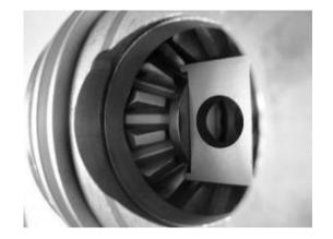
Push axles in and install the c-clips, once this is done pull axles out some until they are properly in place
