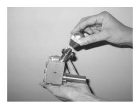
When installing the knob, don't thread all the way down. Make sure that the shifter can shift clear.
