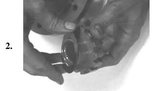
Install thrust washer behind locking side gear.
