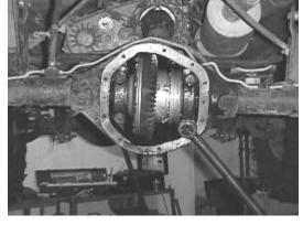
Torque bearing caps to 80 FT LBS. Install axles, rotors, brakes, and tires in accordance with your MSM.
