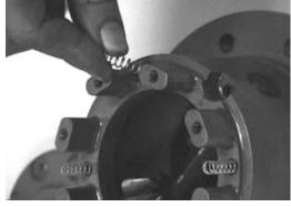
Install the 4 springs in the 4 chamfered holes.
