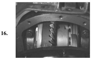
Install cover on to the differential. Make sure the fork slides on the locking ring.
