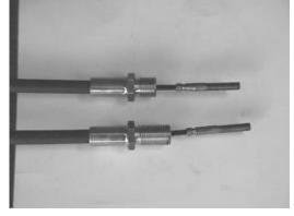
The cable has a short fitting and a long fitting. Short fitting goes into the cover.
