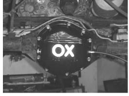
Install diff cover bolts supplied and torque to 30 FT LBS. Note: Use gasket or sealant in accordance with your MSM.
