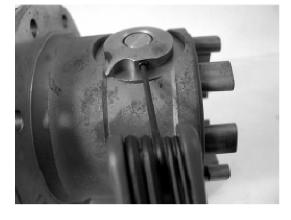
Install the dowel pin an then the set screw. Add High Strength Lock-tite to the set screw prior to installation.
