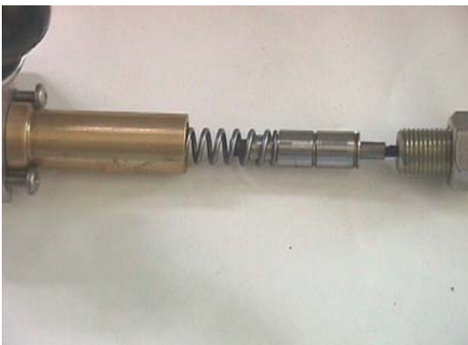
Place spring on piston and into the swivel fitting on the shifter.
