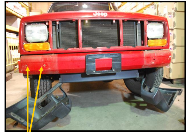
Remove 2 Screws For Vacuum Canister Here
