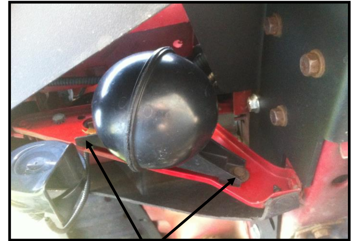
Drill Holes and Fasten In These Locations
