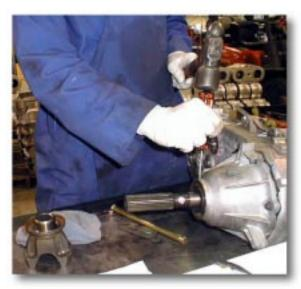
(Fig. 5) Rear Seal Removal
