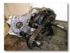
(Fig. 11) Front Drive Chain & Shaft Removal
