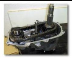
(Fig. 5A) New Main Output Shaft Assembly
