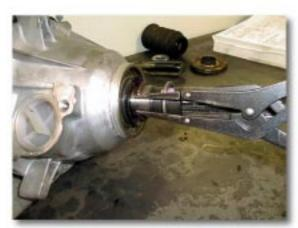
(Fig. 4) Stop Spacer & Snap Ring Removal
