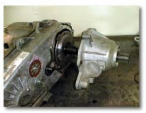
(Fig. 8) Rear Tailhousing Removal
