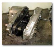
(Fig. 9) Rear Case Half Removal
