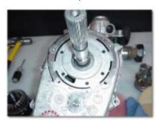
(Fig. 10) Oil Pump Removal
