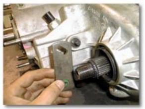
(Fig. 2) Range Selector Removal
