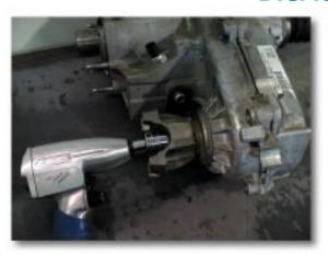
(Fig. 1) Yoke Nut Removal
