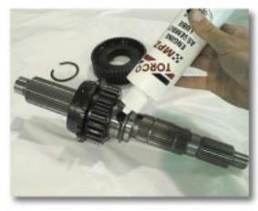
(Fig. 3A) New Main Output Shaft Assembly
