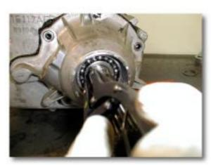
(Fig. 7) Rear I.D. Snap Ring Removal
