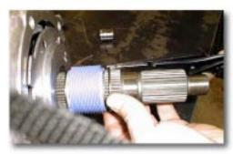
(Fig. 9A) Speed-o- Ring Gear Install
