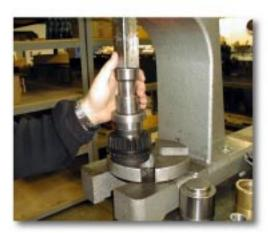
(Fig. 2A) Pull the Needle Bearings Out
