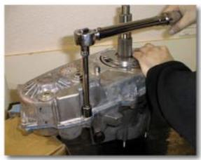
(Fig. 8A) Case Halves Assembled
