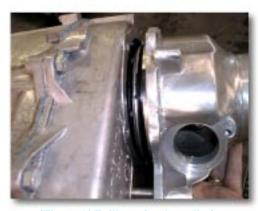
(Fig. 12A) Tailhousing Installation
