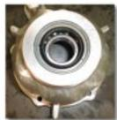
(Fig. 11A) Seal Installed
