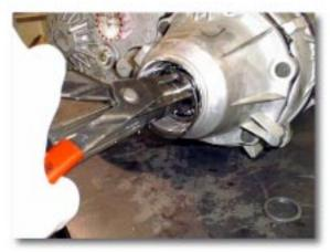
(Fig. 6) Rear O.D. Snap Ring Removal
