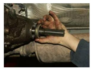
Using lock ring pliers remove the retaining ring that holds the output bearing in place on the factory output shaft.
