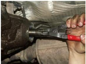
Then remove the speedometer drive gear assembly, unplug the 3 wire connector, remove the bolts that secure the output housing to the transfer case, and remove the output housing
