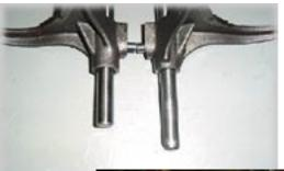
**Note:** Verify the length of your mode fork shift rod as shown. If your shift rod measures 10.2", it will need to be cut down to a length of 9.380". This is typical of 1988 and 1989 model YJ's.
