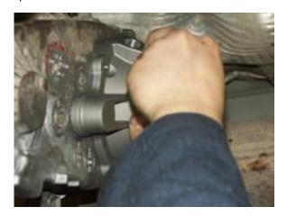
The bearing, snap ring and oil seal should be already installed in the new rear output housing when you receive it from your TeraFlex dealer. Clean the mating surface on the transfer case and apply RTV sealant. Install the new rear output housing and retaining bolts.
