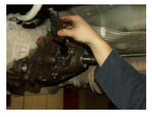
Next remove the bolts that hold the case halves together. There are different style fasteners used here so pay attention to which bolts go in which holes for reassembly.
