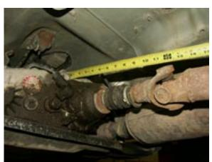
There are a couple of different styles of output slip yoke and housing on 231J transfer cases. The photo to the left is typical.
