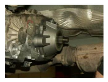
Install the speed sensor in the hole of the new tail housing. Use a little oil on the o-ring to ease installation. Install the retaining bolt and carefully tighten it to secure the sensor. No more than 7 ft. lbs. to avoid damaging the sensor.
