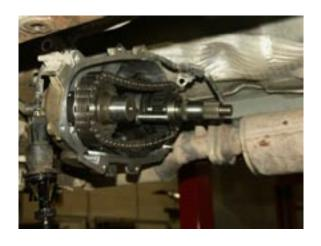
Reinstall the lock ring, then place the new output shaft assembly back into the drive chain and prepare to reinstall the drive train back in the front case half by cleaning the case half mating surfaces
