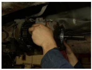
Next, carefully remove the output shaft, the front output gear and shaft, the drive chain and shift fork all together as an assembly and lay them on a clean workbench. Pay attention to the coil spring on the shift fork shaft. You will need to put it back on the shaft before assembling the back half of the transfer case.
