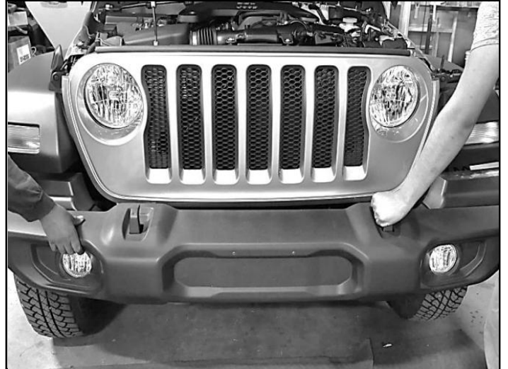
Step 6. With help from an assistant firmly pull the front bumper off the frame rails and set it aside in a protected area.
