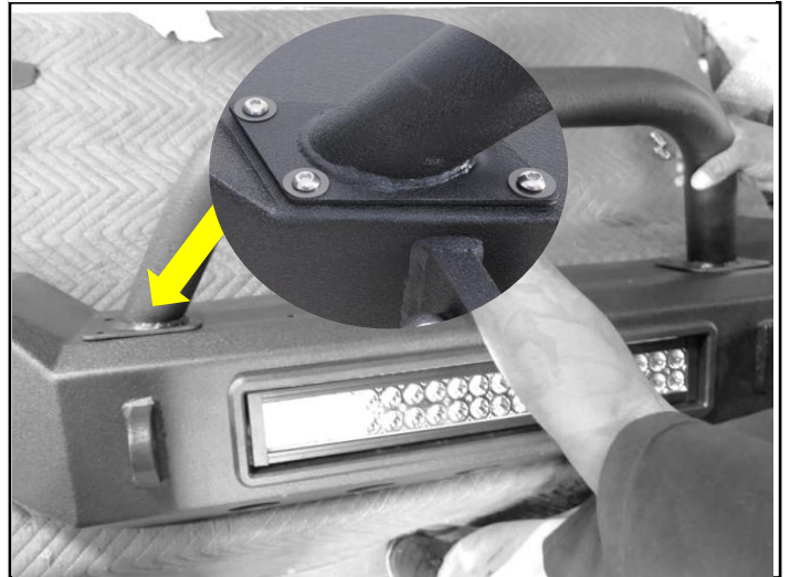
Step 2. Place allen head bolt M8x1.25x25mm and nylon washer through the holes in the bumper cross bar and through the bumper holes. Place a supplied M8 flat washer with supplied M8 split washer onto the end of bolt. Start a supplied M8x1.25 hex head nut at the end of bolt. Tighten down using a 5/32 allen wrench. Repeat step for remaining bolts. Repeat step for other side.
