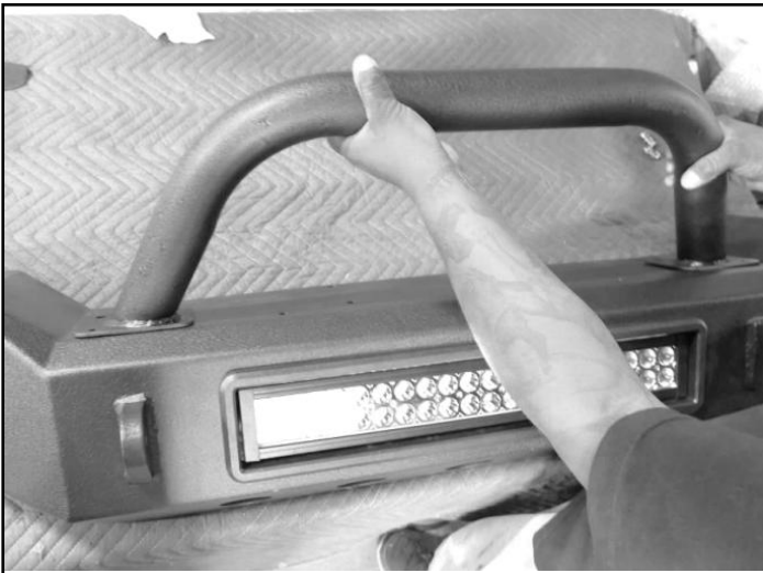
Step 1. Working on work bench. Install supplied bumper hoop onto bumper as shown. Line up the holes in the hoop with the holes in the bumper.
