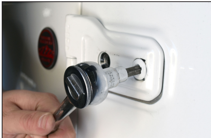
PIC 01: Remove the OE hinge bolts.
