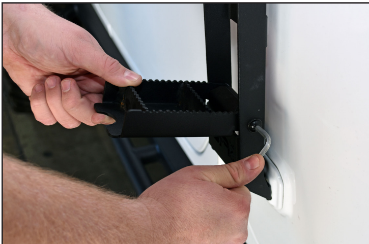
PIC 04: Adjust step pivot tension.
