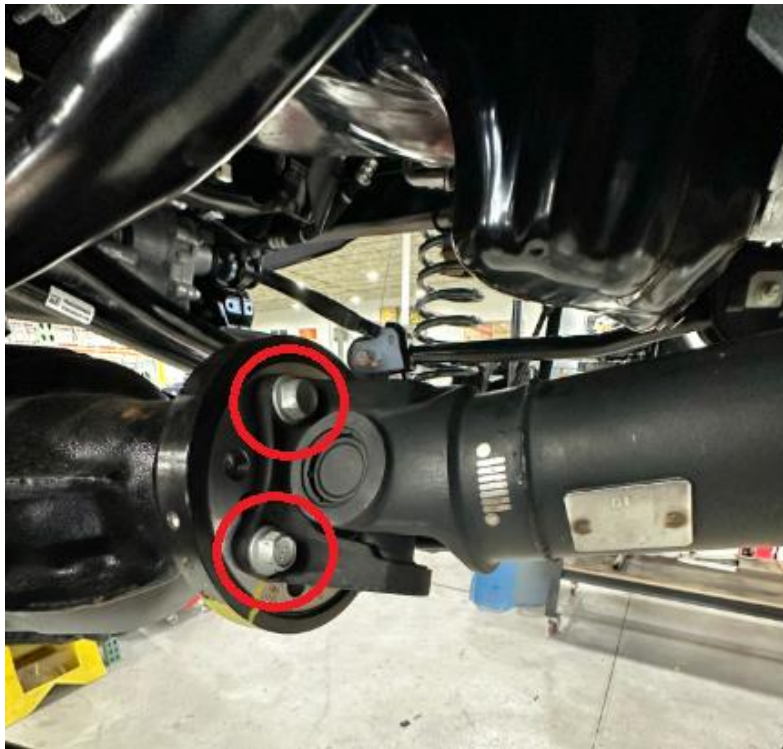
Image 1: Drive shaft bolts
