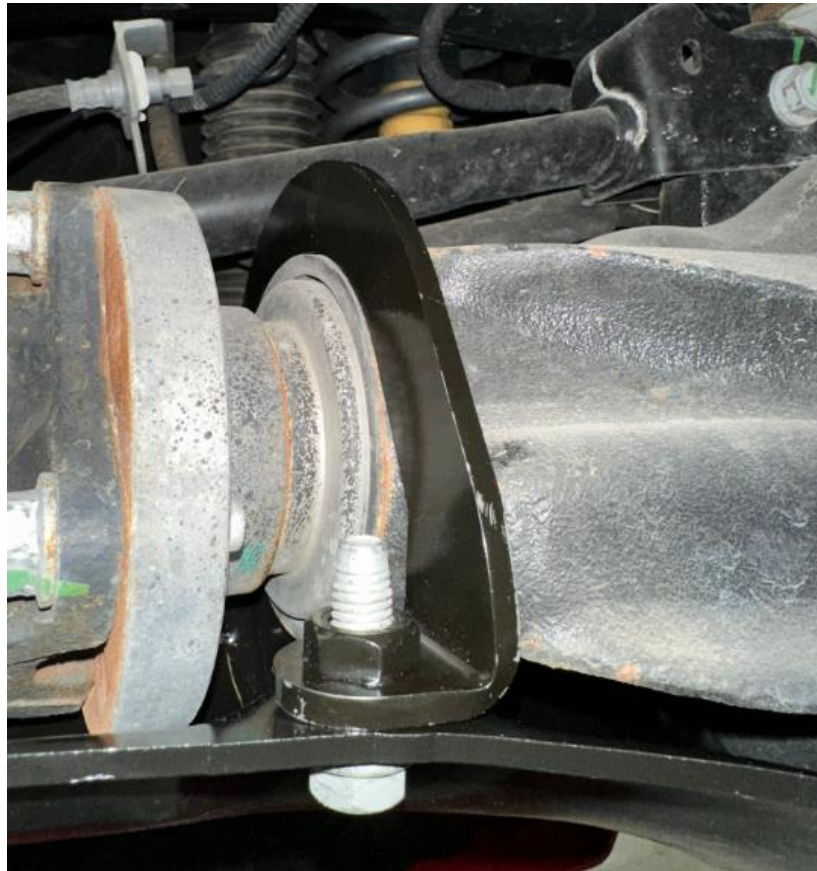
Image 5: Differential Slider Bracket Install
