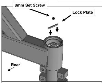
(Fig 17) Once Castle Nut is properly adjusted, slide Lock Plate down into slot in Spindle. Secure Lock Plate to Spindle with 8mm Set Screw
