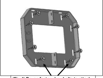
(Fig 4) Reuse factory hex bolts to attach the Tailgate Mount Bracket to the tailgate
