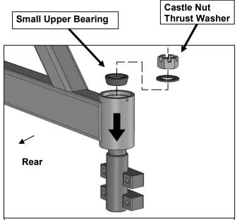
(Fig 16) Slide Swing Arm down over Spindle.
