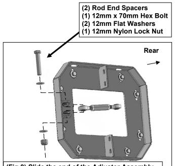
(Fig 8) Slide the end of the Adjuster Assembly between the Rod End Spacers. Attach Adjuster Assembly to tabs and Spacers
