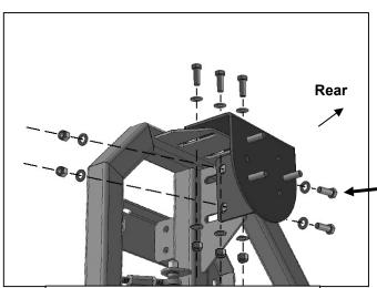
(Fig 21) Attach Tire Mount to top and left side of tabs on Swing Arm
