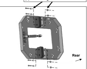
(Fig 9) Attach the Rubber Bump Stops to the Tailgate Mount. Spacers illustrated (arrows) are used for adjustment between the Swing Arm and the Bump Stops only as needed (see Fig 16)
