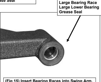
(Fig 15) Insert Bearing Races into Swing Arm. Apply Grease to Lower Bearing. Insert Lower Bearing into Race. Install Grease Seal
