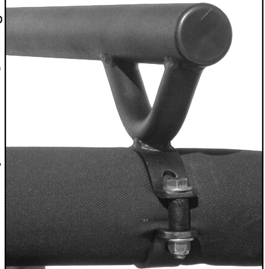
Rear cross bar installed
