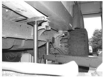
3. The factory body bushing will need to be cut to allow the Rocker Guard to be mounted between the body mounts and the cab of the Jeep. Measure, mark, and cut 3/16" from the top of the bushing. Replace the body bushing and hardware back onto the Jeep leaving the hardware loose SEE PHOTO BELOW AND IN NEXT COLUMN.
