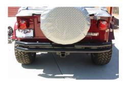
3) Locate the rear bumper onto the mounting brackets and attach through the top and bottom of the brackets with 8- 12mm bolts, flat washers, lock washers and nuts supplied. Tighten to 45lbs torque.
