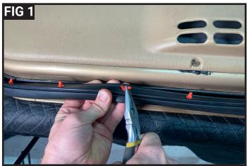
Put on Safety Glasses. Remove original door seal by removing from door surround channel or by pulling out door seal clips. Re-install new door seal by working the seal into the door surround channel or inserting all the corresponding door seal clips into thier holes in the door.
