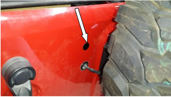
31. Clean area around holes in tailgate. Cover holes in tailgate using the two sticker plug covers supplied in the kit.
