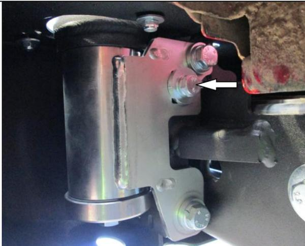
16. Install pivot bush locking bolt assembly.
