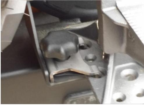
33. Install Hi-Lift clamp plate. Use M10 Knob, M10 Nyloc Nut and Hi-Lift Lock Down Plate.
