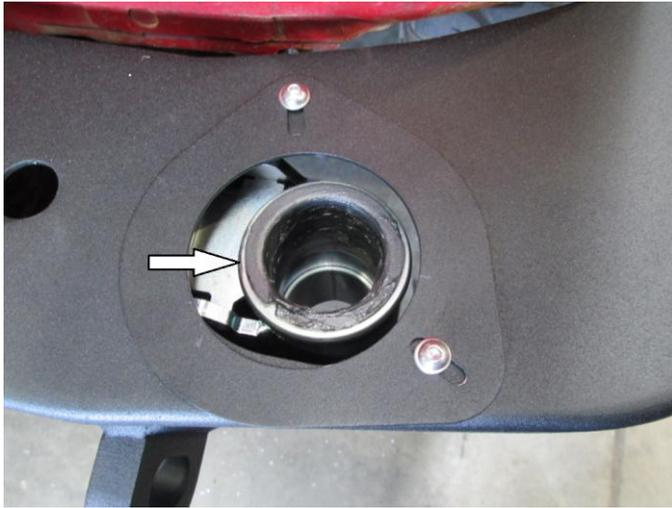
9. Lightly grease pivot bush bore and top face.
