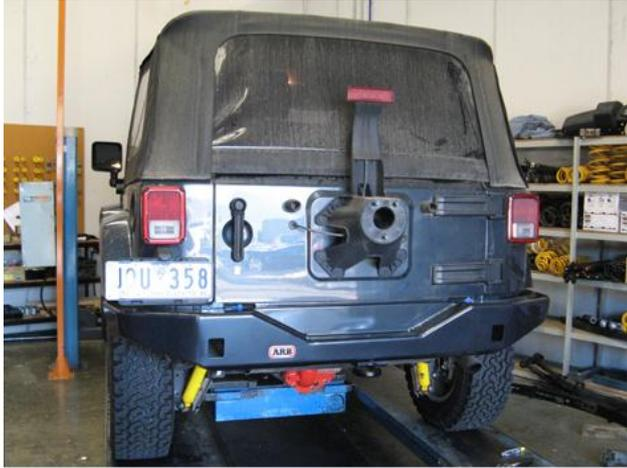
6. Fit (Re-fit) Rear bar to vehicle as per fitting instructions (Part No. 3789186) Steps 7 – 14.
