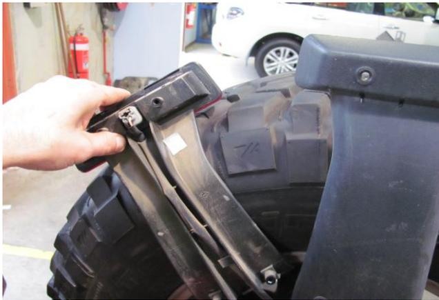
7. Remove O.E. wheel holder from vehicle and retain all components. Remove and un-plug stop light housing.
