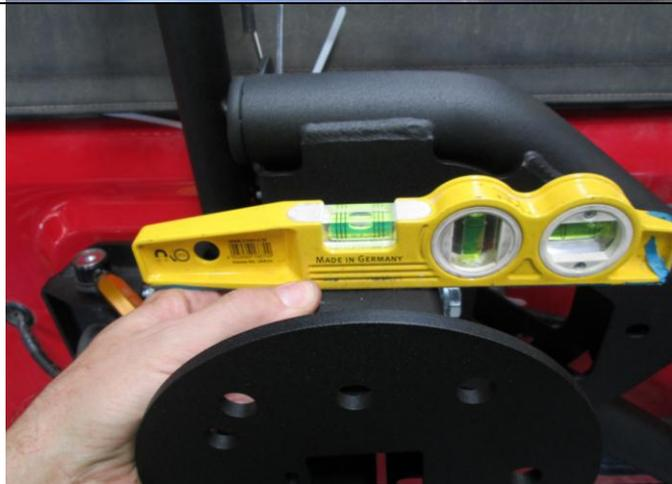
14. On level ground, use a spirit level or similar to level the Carrier Arm.
