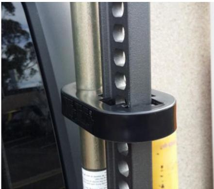
34. Install handle keeper (Part No. ARB203HKB/ARB203HKR) to Hi-Lift jack to eliminate handle rattle.
