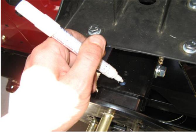
29. **Move wheel mount inwards approximately 10mm.** This will place some load on the tyre when all is secured. Mark bolt hole position, drill to 10mm and secure using M10 SEMS bolt and M10 flange nut. Tighten M10 bolt first followed by side bolts to specified torque.
