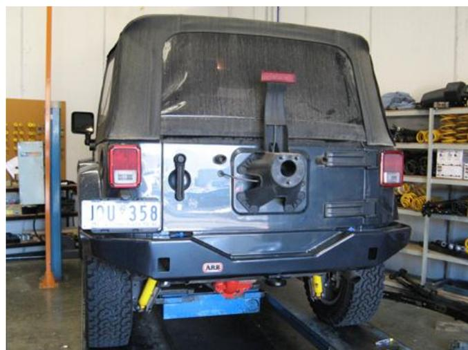
1. If vehicle is already fitted with ARB Rear Bar (Part No. 5650360) remove in reverse order of fitting instructions (Part No. 3789186 - stopping at step number 5). If ARB Rear Bar is not yet fitted carry out steps 1 – 5 from Fitting Instructions (Part No. 3789186).
