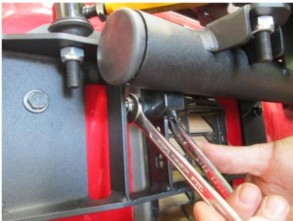
17. Install Carrier Arm Stop using M8 x 40 Bolts, M8 Flat Washers, Plate Washer and M8 Nyloc Nuts.
