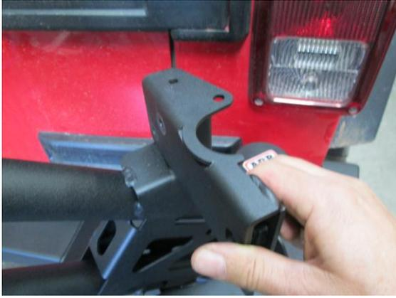
21. Install Hi-Lift bracket. Use Bolts M8 x 20, M8 Spring Washers, M8 Flat Washers and M8 Flange Nuts. Do not tighten fully.
