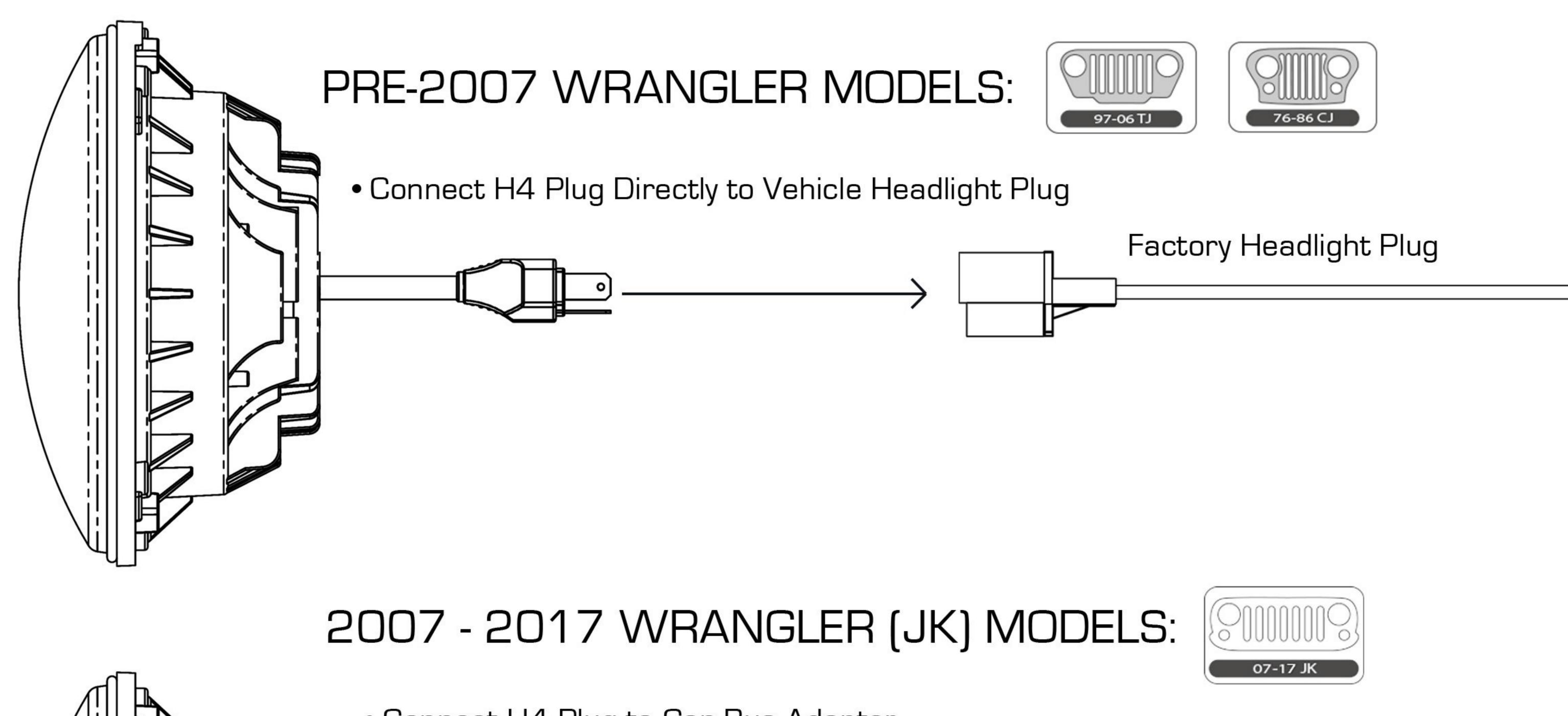
Connect H4 Plug to Can-Bus Adapter • Connect Can-Bus Adapter to H4/H13 Adapter
