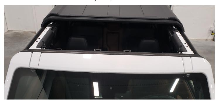
2. Remove the Velcro strip from the foam seal and attach to the vehicle above the door frame.
