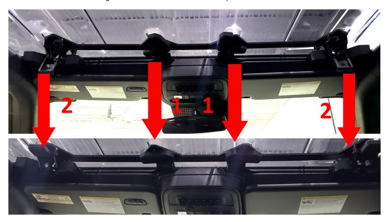
6. Turn the Rear wing clamps starting with the center two clamps.
