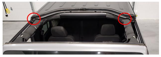
2. Place the clear roof panel on the top of the vehicle. Do not remove the protective film from the clear roof panel until the installation is complete. Only peel back the protective film as far as necessary to install the clear roof panel.
