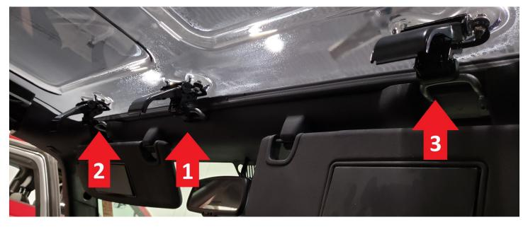
6. Starting at the rear of the vehicle, slowly tighten the hand bolts in the order shown below. Do not over tighten.
