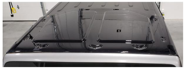
3. Align the clear roof panel with the rear stock roof panel by lifting the panel and pulling towards the rear of the vehicle. A properly aligned top should look like the pictures below and aids in threading the stainless steel hand bolts into the nut plates.
