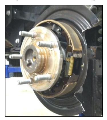
Figure 3: 3/4 view of the dust shield trimmed for caliper clearance
