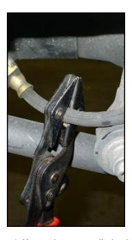
Figure 1: Hose crimpers applied to brake hose
