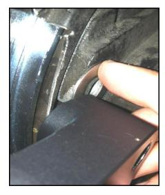
Figure 7: Shim placement between the caliper bracket and axle housing end
