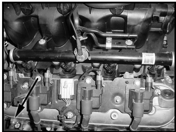
Figure 13 Passenger Side Coil Connection
