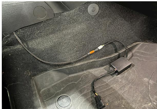
Fig. 13: Connect Controller to Switch Harness.
