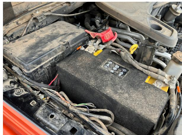
Fig. 33: Connect battery ground cable and GND\_BATTERY ring terminal.
