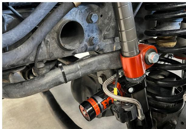
Fig. 28: Connect harness to QSE-Link mating connector.
