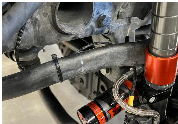
Fig. 26: Route the driver side Link Harness.
