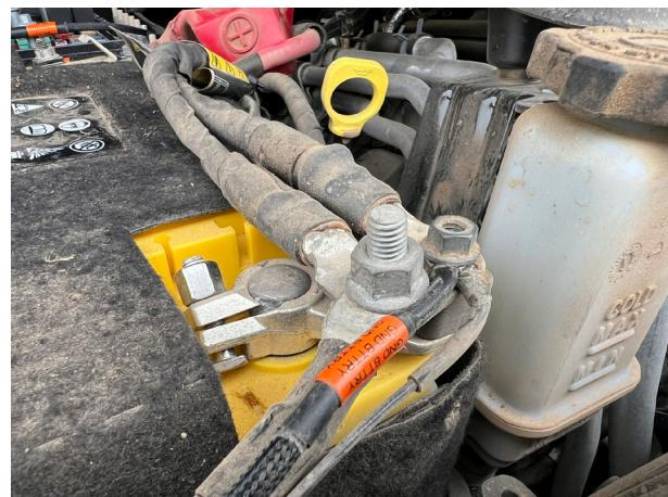
Fig. 34: Connect battery ground cable and GND\_BATTERY ring terminal.
