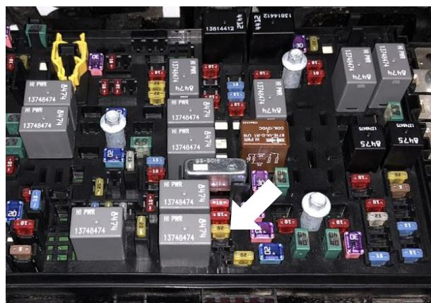
Fig. 29: Remove the yellow fuse from the fuse box.
