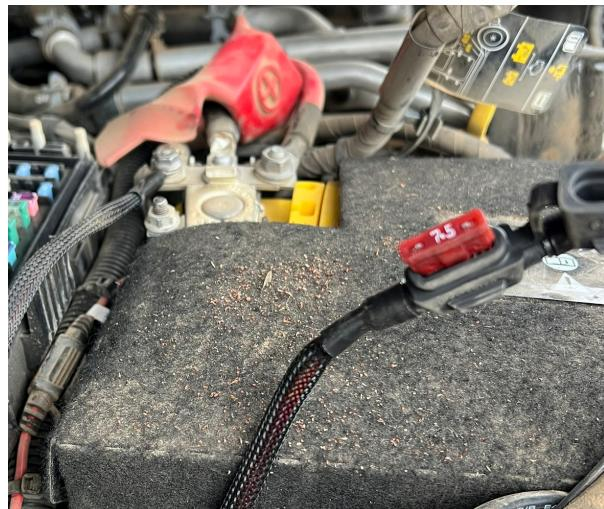
Fig. 32: Install the fuse in the fuse holder.
