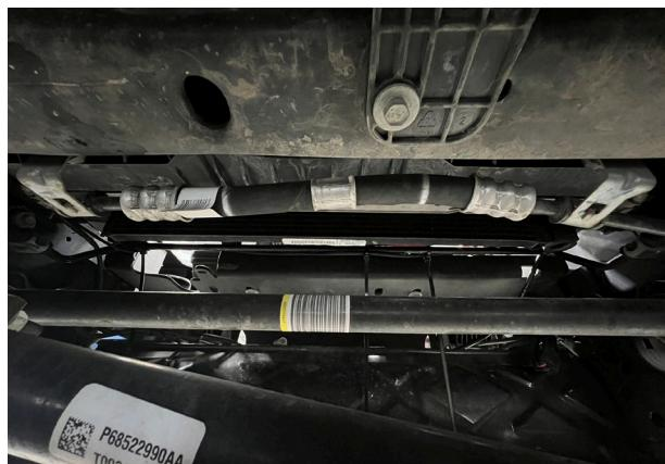
Fig. 25: Route the driver side Link Harness.
