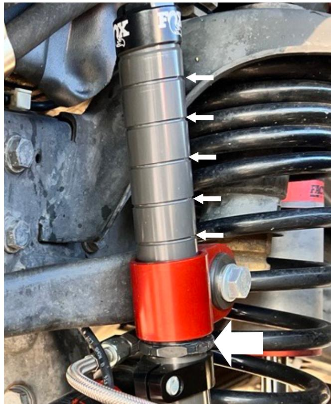
Fig. 5: Grooves (upper small arrows); eyelet nut (lower large arrow).
