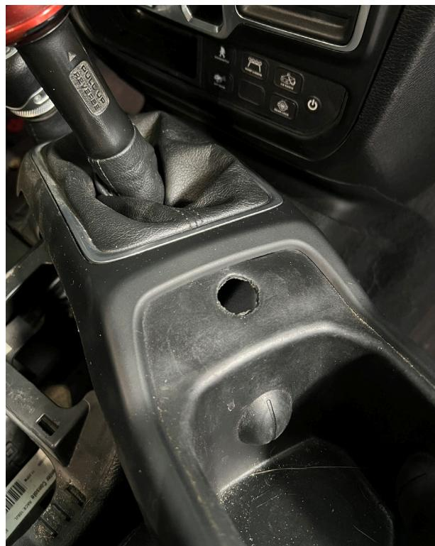
Fig. 8: Drill a hole in the cup holder trim.
