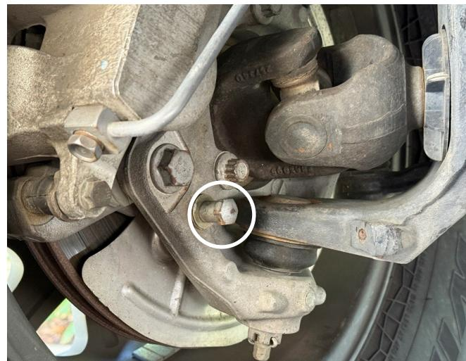
Fig. 3: Torque steering stop/spacer assembly (circled area).
