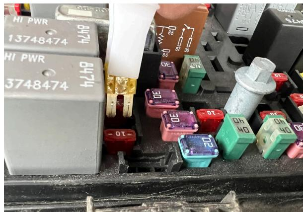
Fig. 30: Remove the yellow fuse from the fuse box.
