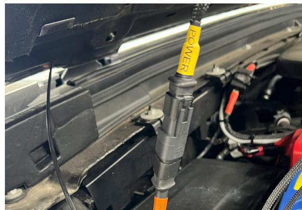
Fig. 21: Connect 3-pin connector to Link Harness.
