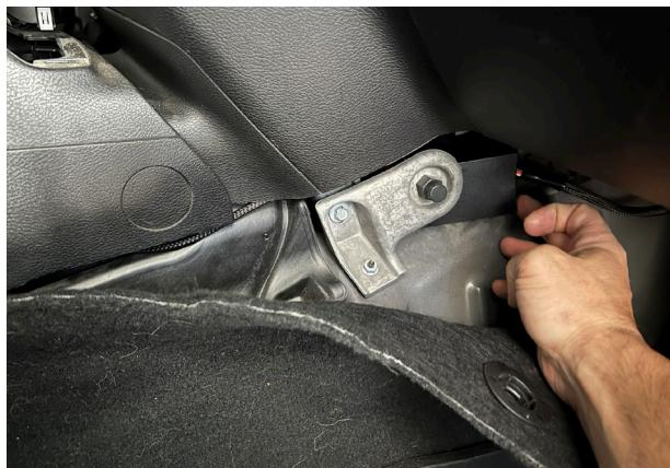
Fig. 14: Lift the carpet to route Controller Harness.
