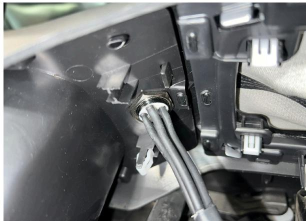
Fig. 11: Secure the switch in place.
