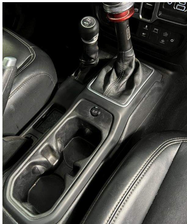
Fig. 35: Reinstall the cup holder/shifter trim.
