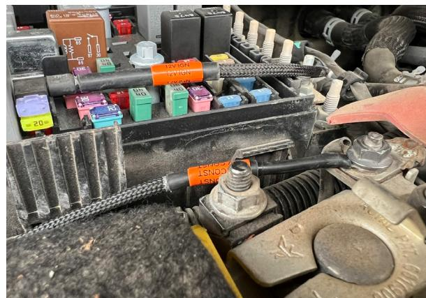
Fig. 31: Install the Micro3 tap into the lower slot and the 5A fuse into the upper slot; install Micro3 tap into empty slot for fuse #F52; connect two terminals.
