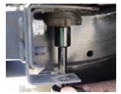
Locate the left and right bumper mounting brackets. Place left bracket with large vertical tab facing outwards, towards the inside of the vehicle. Align inner and outer mounting holes with the rear frame cross member. (2 outside of frame rail, and 2 inside frame rail for each side). Use the 10mm bolt washer, and nut. Torque bolts to 50 ft-lbs.
