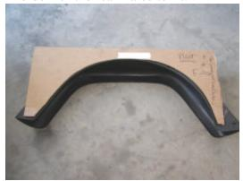
This cardboard pattern provides an outline of how the YJ rear wheel opening needs to be modified. Just be sure to properly mark the front and back and the proper orientation (left and right) before making any cuts.
