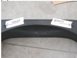
It is necessary to remove the two (2) locating studs from the rear flares. The studs are only used on TJs, and are not used on YJs. Carefully remove these studs.
