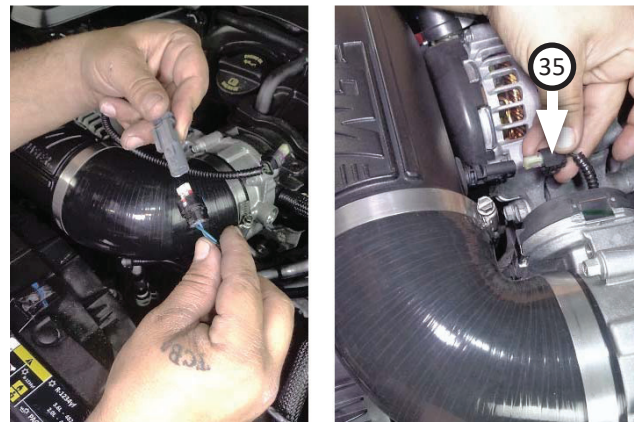
34. Connect air temp sensor extension harness (35) to vehicle's temp sensor plug. Route lead under coupler, connect other end to air temp sensor, then make sure all connections are secure.
