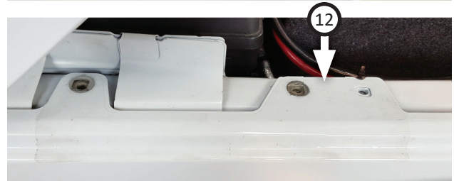
21. Remove bolts (x2) from fender beside fuse box. Then align hood gasket (12) with bolt holes (x3) on fender and press it on, working out air bubbles.
