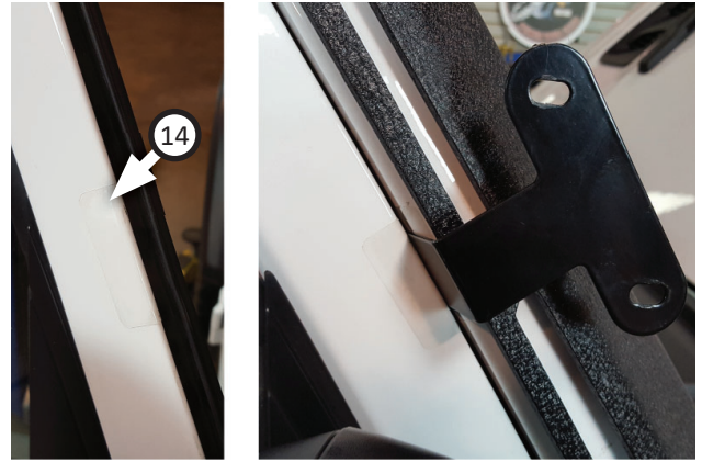
27. Carefully close passenger door, align door gasket (14) on outside so it protects door from rubbing against bracket 3 then apply it to front/inside.
