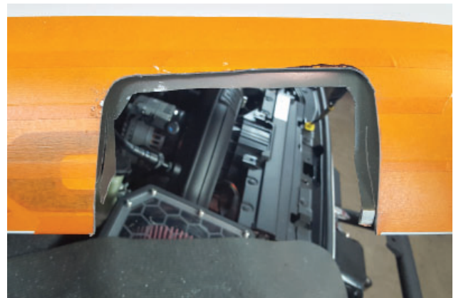
46. Make another cut up to your marks through top layer. Use a file to smooth your cutout so you can more accurately compare its location to tube.
