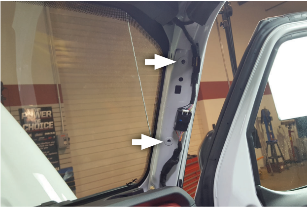
24. Remove bolts (x2) securing grab handle to A pillar, and set parts aside for later use.
