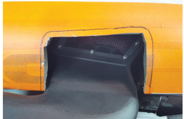
45. Make another cut closer to marks on cutout. If you have to move your cutout one way or another, this is the best time to do it.
