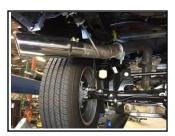
**6.** Remove the rear factory rubber insulator. Install the exit pipe #D onto the overaxle pipe and attach with band clamp# E. Re-install the factory rubber insulator. Do not tighten.
