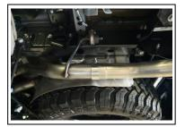
7. Lastly, install exit pipes (F) and tips (L) onto both Driver side and Passenger overaxle pipes. Position the exit pipes to what meets your expectations.
