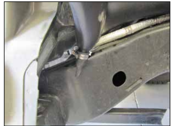
58. Install the duck bill fitting onto the port at the bottom of the corner tube and secure with the provided hose clamp. NOTE: be sure all of the hose clamps securing the corner tube are turned in such a way that they will not interfere with the fender once it is installed.
