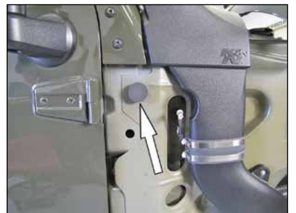
59. Peel the backing of the provided damper pad and then install it as shown on the inner body. NOTE: Be sure all of the hardware is secure before moving to the next step.
