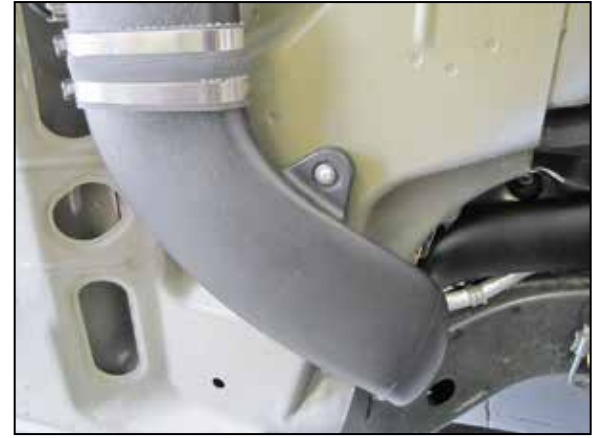
57. Secure the corner tube with the provided sheet metal screw into the hole previously drilled.
