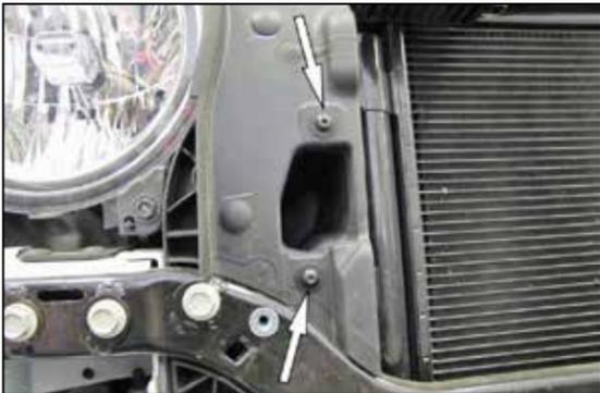
8. Remove the two bolts that secure the inlet scoop to the core support and remove inlet scoop.
