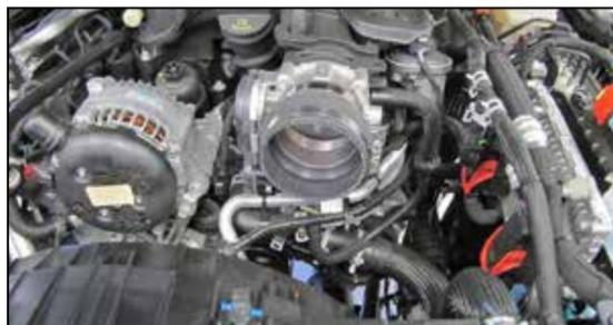
16. Install provided hose onto the throttle body (08171) secure with provided clamp.
