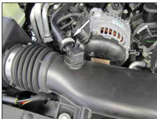
3. Disconnect the crank case vent line.
