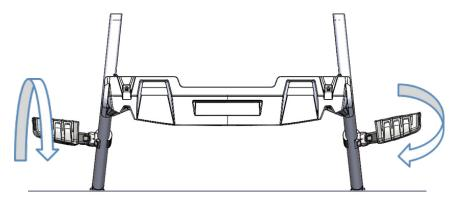
Rotate mirror body and adjust the forward/backward sweep of the break-away joint.
