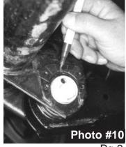
10. Remove and replace the lower links with new Skyjacker extended links (one side at a time). On Grand Cherokee models, mark original position of eccentric cams (see photo #10). Do not tighten bolts until both sides are installed (see photo #11). On Grand Cherokee models, set the eccentric cams back in original position.
