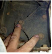
Disconnect the vapor bottle on the passenger side and allow to hang to the side for now.
