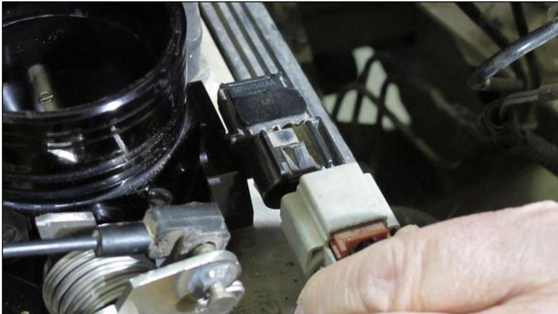
**(Figure 23)** Reconnect the MAP Sensor connector as shown above .
