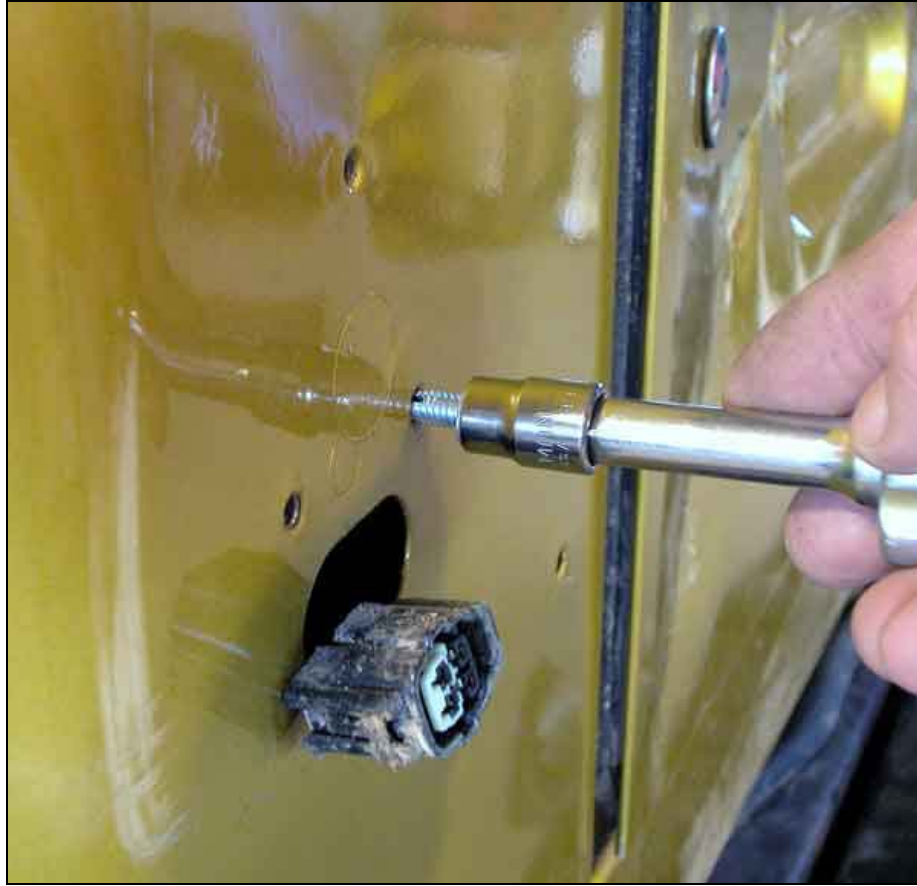
Image 7 - Threading body with self tapping screw
