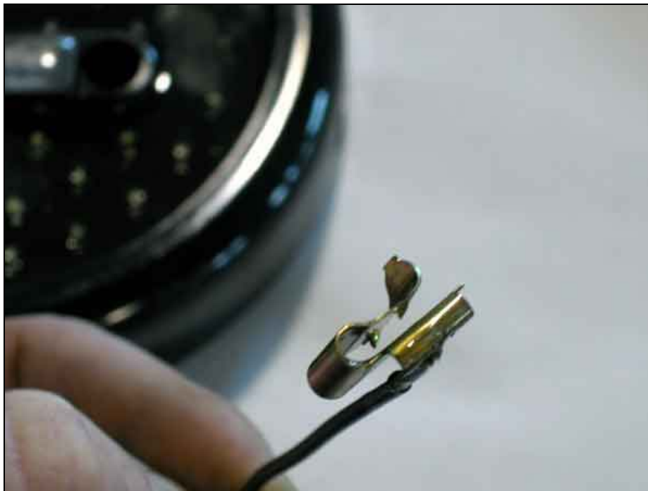
Image 9 - Paint Piercing Ground clip, slide sharp fangs over painted edge of body seam
