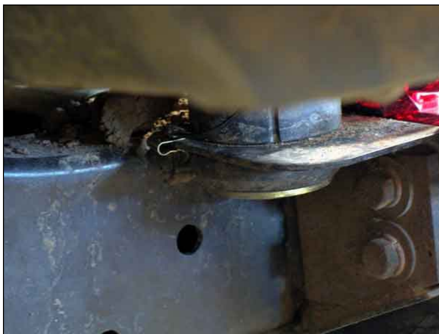
Image 10 - Example ground tab mounting location
