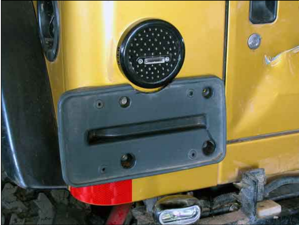
Image 13 - Example of License Plate trimming if OEM plate bracket is reused
