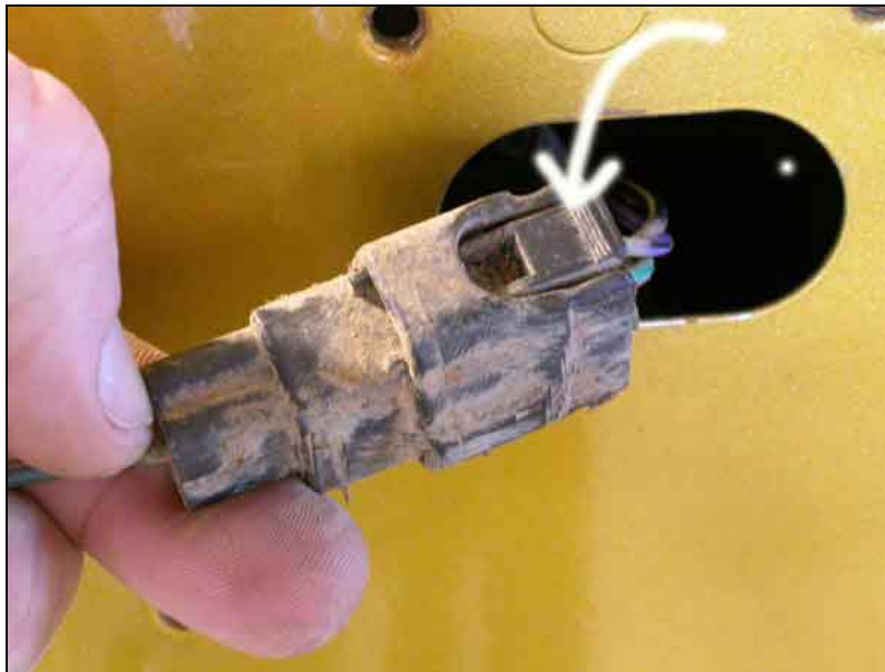
Image 3 - Press this tab to release connector
