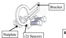
Ref. "B"- (1) Throttle Cable Bracket (2) 3/8 ID x 3/4 OD x .636 Spacers (1) Nutplate with 3/8-16" threads (2) 3/8-16"x 1 1/2" Hex Head Bolts
