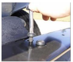
After the new bumper has been installed on the front of vehicle, hand tighten all bolts into place. Using the Star bit tighten all bolts to secure bumper to frame. If installing new tow hooks used supplied hardware for upper mounting holes.
