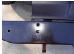
Note: Please keep all mounting bolts as they will be reused. A size 55 star bit will be needed to remove original mounting bolts from vehicle.
