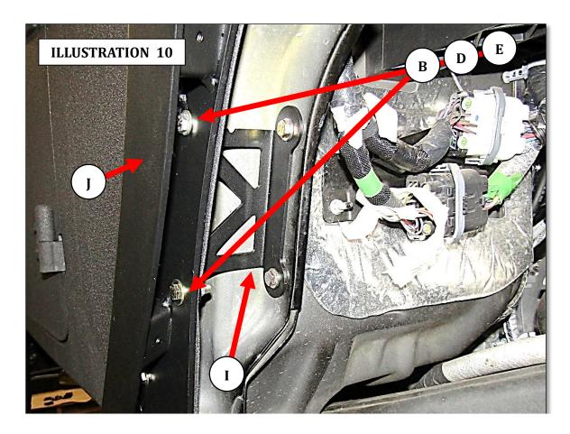
**Step-12** Attach the remaining holes in the Trailline fender to the vehicle body panel using the supplied  $\frac{1}{4}$ " x 1" hex bolts, flat washers and locking hex nuts.
