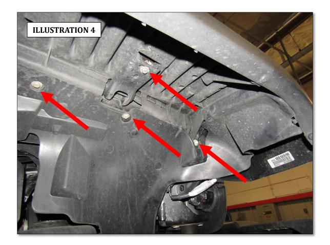
**Step-5** After you've removed the OEM fender clip fastener and bolts, grab the fender, lift it up and pull outward from side to side while wiggling it. Continue to do so gently until it comes off. Remove any plastic clips that may have broken off and remain in the holes on the vehicle body.
