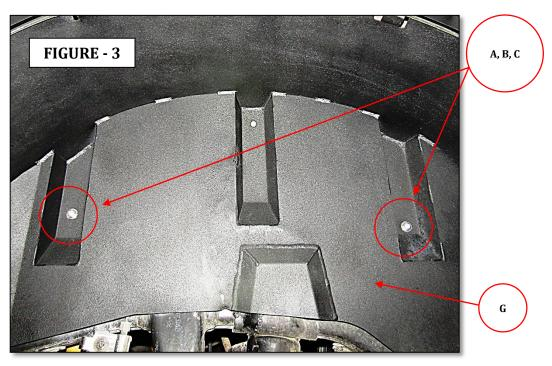
**Step-7** Align the (2) threaded tabs at the top of rear inner fender liner with the holes in the OEM fender body panel, and secure the rear inner fender liner to the body panel using (2) ¼" x 1" button head bolts, (2) ¼" lock washers and (2) ¼" flat washers, (FIGURE-4). Leave the bolts loose for final adjustment.
