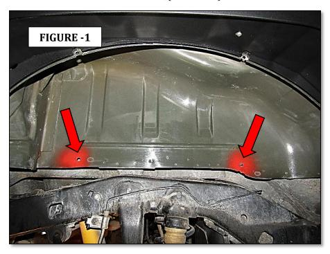
**Step-4** Enlarge the (2) holes in the wheel well used for attachment of the OEM fender to 17/32", and Install a  $\frac{1}{4}$ " Rivet-Nut in each hole using the installation tool supplied.
